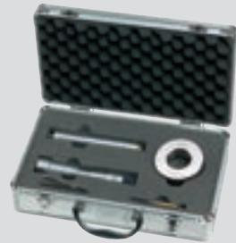
For measuring holes. With friction device that gives a constant measurement force and self-centering measurement device. Measuring faces of hard metal. Measurement tips reach to 0.5 mm from the bottom of a blind hole. Setting ring included.
