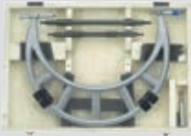
Enamelled low weight frame of steel. Matt chromium-plated scale. Adjustable measuring rod with fixed spacing sleeves. Hardened spindle 8.0 mm with fine-polished measuring faces of hard metal. DIN 863.
