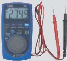
Digital multimeter in pocketsize with autorange. Measuring DC/AC voltage, resistance, frequency and capacitance. Also diodetest, continuity with buzzer, datahold, relative mode, low battery capacity warning and auto off after 15 minutes.
