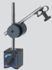
With fine adjustment. With magnetic base. The bottom and back are magnetic. The magnetism is switched on and off with the button. Vertically and horizontally adjustable. Supplied with top and bottom holder, but without dial indicator.
