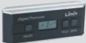
Digital spirit level and angle gauge. Magnetic with V-groove on the base. Can be reset in all positions. Absolute function, which means that the value can shift between the actual 0-value and a second 0-value. The measurement can be frozen in the desired position. Automatic switching off.
