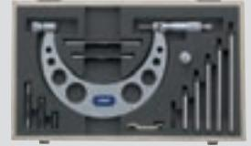
Forged frame. Hardened spindle and interchangeable insert rods 8 mm with fine-polished measuring faces of hard metal. Absolute/incremental measuring. Adjustable absolute value. Friction sleeve and lock nut. DIN 863. Battery type SR 44, art.no. 2928-1003.
