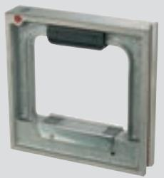
Precision level of cast iron. Adjustable, graduated longitudinal and transverse vials. Precision in accordance with DIN 877. V-groove in contact surface.
