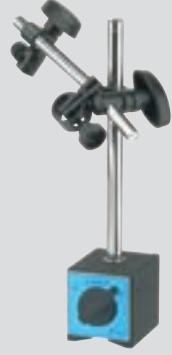
With fine adjustment in the top holder. Holder with holes for indicator dial and dovetail slot for rocker indicator. Central locking with one knob for the bottom, middle and top joints. Magnetic base with V-slot in the bottom. Supplied without indicator dial.
