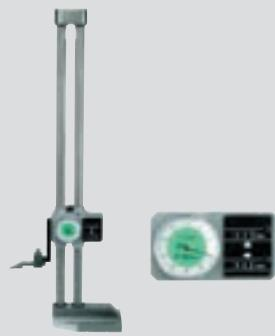
The measurement value is read-off in whole mm on the counter and in 0.01 mm on the dial indicator. 1 pointer turn = 1 mm. Dual counter, one adding and one subtracting, that can be reset individually in optional position. Flexible height setting with knob on the back. Measuring tip of hard metal. DIN 862.
