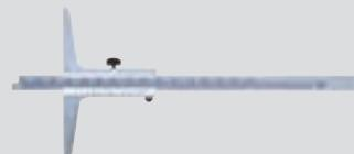
Made of stainless steel. Matt chromium-plated scale. Reversible scale for measuring with hook or tip. Graduated in mm. Vernier scale 0.05 mm. Tolerance according to DIN 862.
