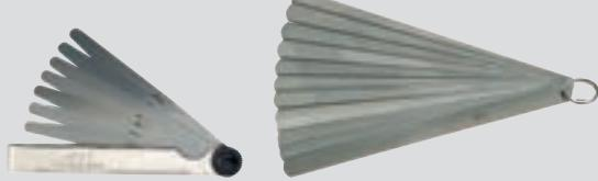
**Calibrated.** Tolerance according to DIN 2275. Certificate included. Calibrated at two measuring points per blade. Blades in mm dimensions. For measuring slots and bearing play, etc. With nickel-plated, lockable holder.
