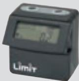
Mini digital level and protractor. The display shows two values. One absolute value and one relative value. Flip up display for easy reading from above. Zero setting in any position. Hold function to freeze the value. Magnet on base for fitting on saw blades, steel frames etc. Automatic off after 3 minutes.
